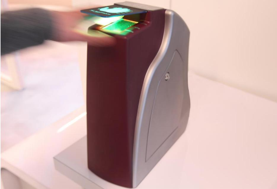
Morpho Finger-on-the-Fly contactless fingerprint reader
