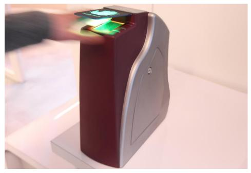
Morpho Finger-on-the-Fly contactless fingerprint reader
