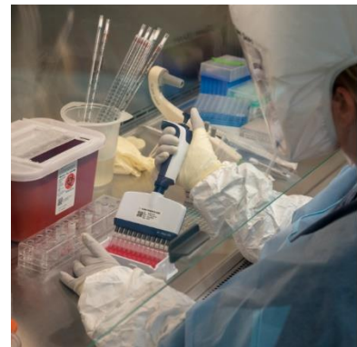
NBACC Scientist working in Biosafety Level 3 containment in a Class II biological safety cabinet performs dispensing of samples using a micropipette, which measures very small volumes of liquid.
